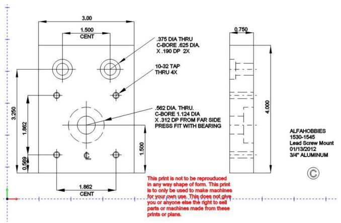
The only tricky part to this part is boring the 1.124 X .312 DP bore to the right size. This bore is for a light press fit of a bearing. Other than that everything else is pretty standard machining. Just watch that you get the bearing bore and the .625 X .190 deep C-bores on opposite sides of the part from each other.
